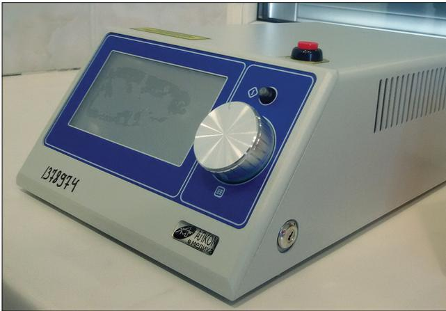
**Figure 6:**The diode surgical laser Alod-01 (wavelength 810-1064 nm, power 1-30 W) used for percutaneous laser intervertebral disc surgery. Used with permission from Barrow Neurological Institute, Phoenix, Arizona
