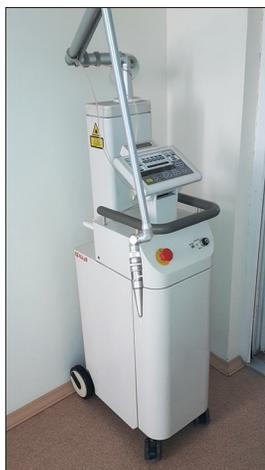
**Figure 2: A CO<sub>2</sub> surgical laser, the UniPulse COL-1040 (Nidek, Hiroshi, Japan), has an articulated arm through which the irradiation is delivered. Five regimens of irradiation effects range from cutting to coagulation. Used with permission from Barrow Neurological Institute, Phoenix, Arizona**
