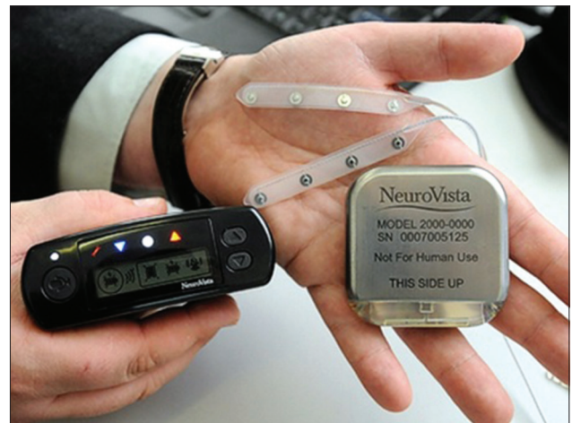
Figure 5: Seizure advisory system: Implanted electrodes (top) (8 of 16 electrodes shown), implanted processor (right), and external patient module (left).
