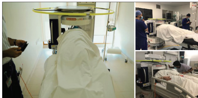
Figure 5: The Swoop® Portable Magnetic Resonance Imaging (MRI) System™ (Hyperfine, Inc., Guilford, CT, USA). This illustration showcases the practical utilization of the Hyperfine Swoop, a portable MRI scanner with low magnetic field strength, within a clinical context. The system's mobility allows it to be transported to a patient's bedside, where it can be connected to a standard wall outlet for power. The operation of the scanner is managed through a wireless tablet. The system boasts a field strength of 0.064T, employs a permanent magnet, and carries a weight of approximately 1400 pounds. On the Left: Connected to a power outlet and used through a wireless tablet. On the Right (Top and Bottom): Use of the system in a practical setting.
